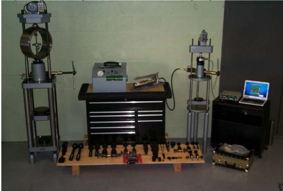
Pictured Left: A typical 10,000 LBF Morehouse Direct Reading Load Cell Calibration System.
