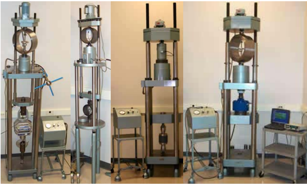
Above: Samples of setups using Morehouse universal calibrating machines.
