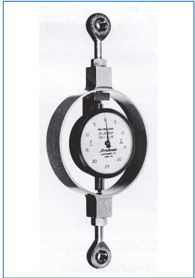
Figure 4. Model 5BT; 50 lbs. capacity Ring Force Gauge with push/pull calibration to 25 lbs. Maximum calibrated load with push/pull calibration is 1/2 capacity.
